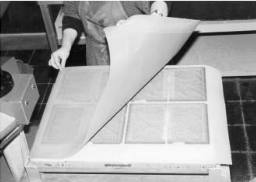
Fig. 2: Putting the second strengthening sheet onto the backside of the leafcast sheets lying on Hollytex
